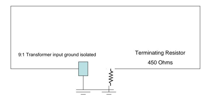
40 Ft Horizontal – 10 Ft vertical – Bottom wire is 18 – 24" off ground. Feed and termination are in middle of bottom wire...(DEAD CENTER)
